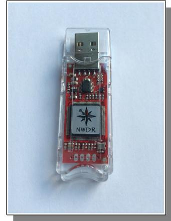
Current products in this space use the older AMBE-2000 series of vocoder chips which do not support additional digital voice radio standards such as DMR, System Fusion, dPMR, NXDN, P25 Phase 2 HR, and others, which can be addressed by the newer AMBE-3000 series vocoder chip as found in the DV3000 and ThumbDV™, pending further 3<sup>rd</sup> party software development.<sup>3</sup>
